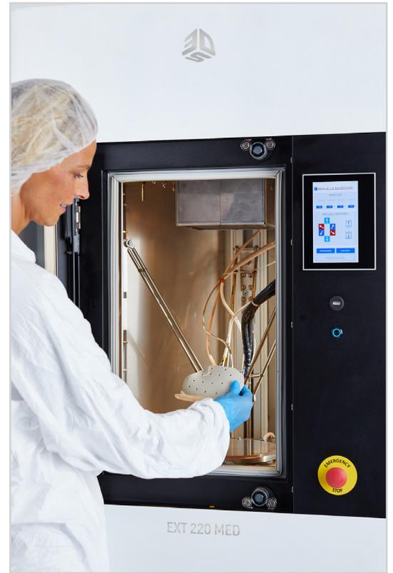
Temperature-controlled chamber with a full build envelope (220mm diameter, 150mm height)
