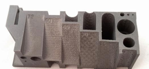
Example of **downfacing surfaces** in different angles ranging from:  $75^\circ$  (left) to  $0^\circ$  (right) with steps of  $15^\circ$
