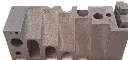
Example of **upfacing surfaces** in different angles ranging from:  $0^\circ$  (left) to  $90^\circ$  (right) with steps of  $15^\circ$
