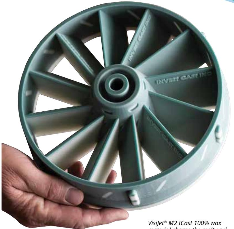
*Visijet® M2 ICast 100% wax material shares the melt and burnout characteristics of standard casting waxes.*
